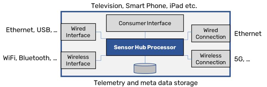
Figure 3 Sensor Network Gateway architecture
